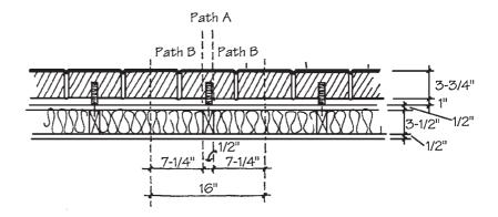
Stud spacing = 16.00 in. o.c., or 1.33 ft o.c. Height of the section = 12.00 in. or 1.00 ft Total area,  $A_t = 1.33 \times 1.00 = 1.33$  sq ft Width of Path A = 1.50 in. or 0.125 ft Area of Path A,  $A_A = 0.125 \times 1.00 = 0.125$  sq ft Width of Path B = 16.00 - 1.50 = 14.50 in. or 1.208 ft Area of Path B,  $A_B = 1.208 \times 1.000 = 1.208$  sq ft
